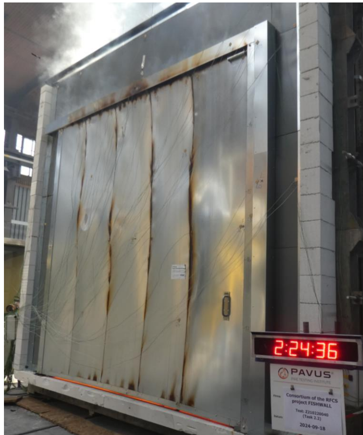
UF after 144 minutes of the test
