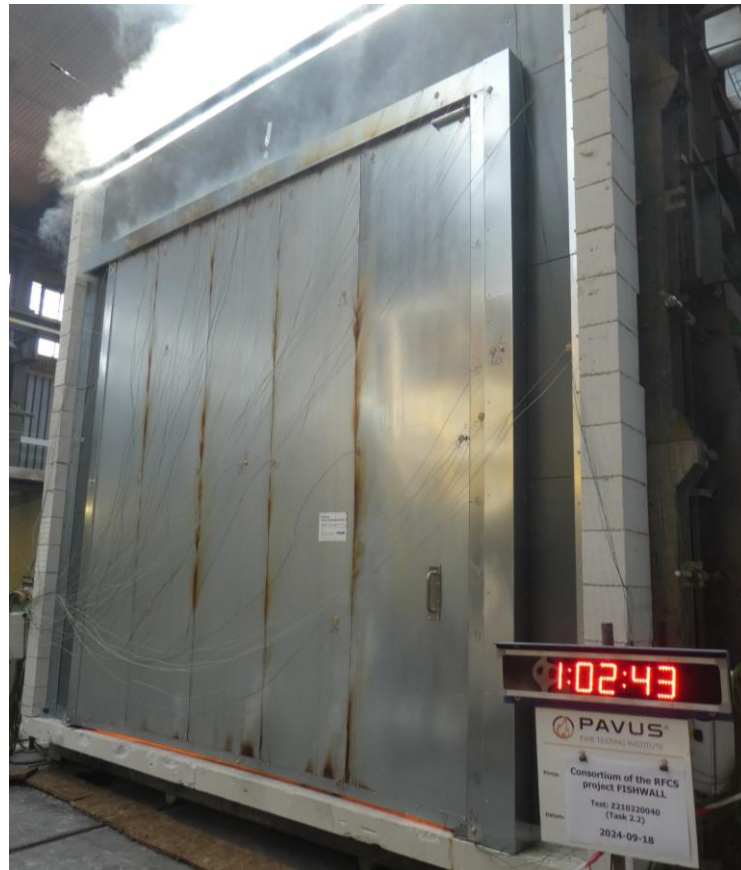
UF after 62 minutes of the test
