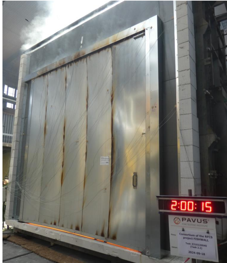
UF after 120 minutes of the test
