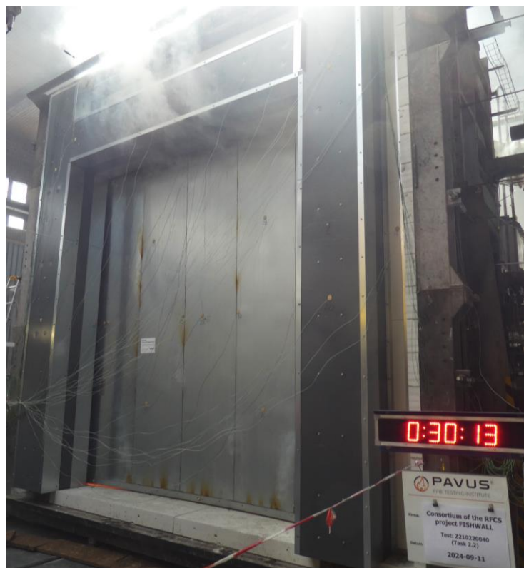
UF after 30 minutes of the test
