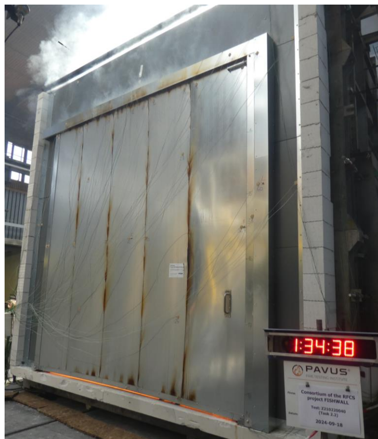
UF after 94 minutes of the test
