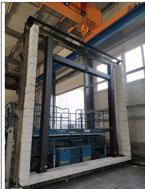
a) View of the support steel frame
