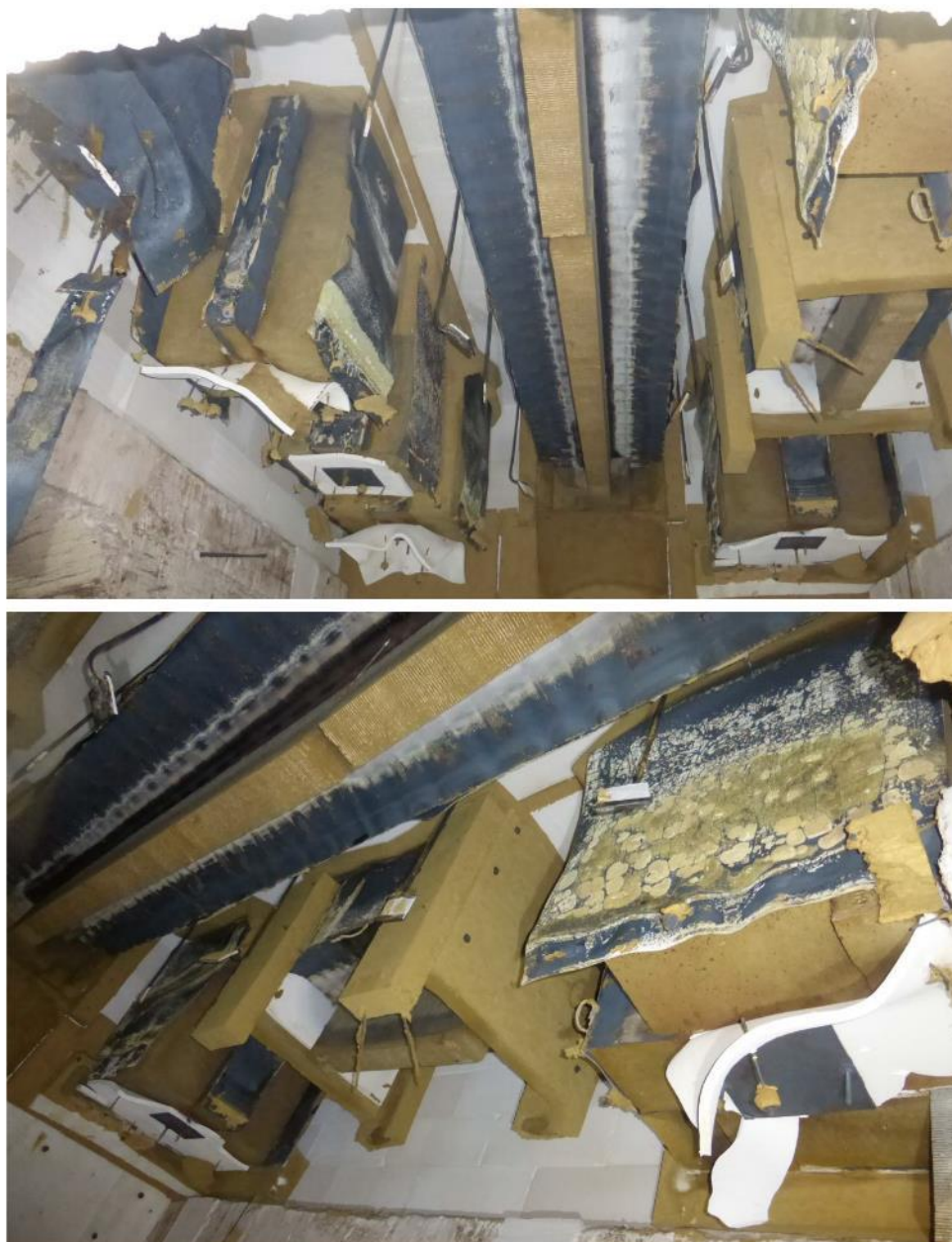
Specimens after the test in the furnace
