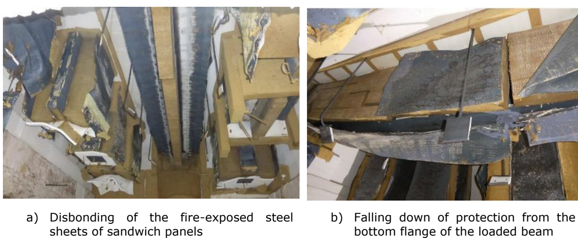
Figure 6: Views of test specimens after the tests
