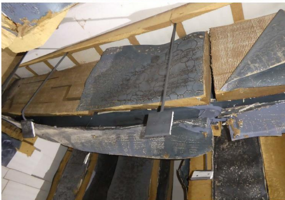
Specimens after the test in the furnace
