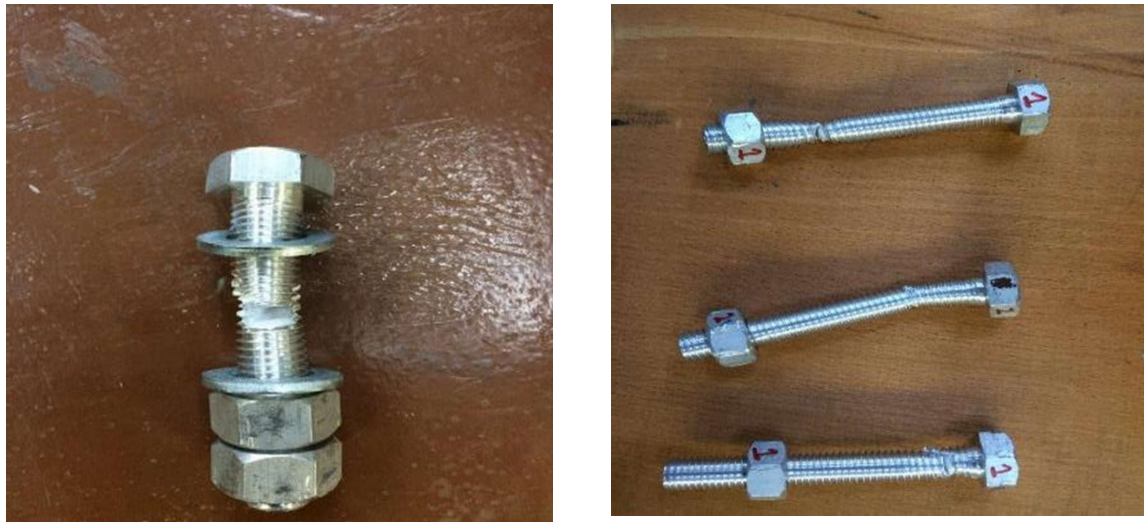
Figure 11: Failure thread destruction of AA6XXX series bolts in tension
