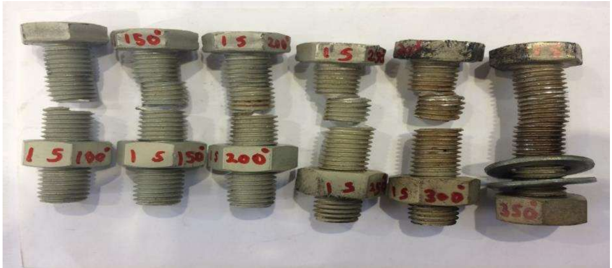
Figure 15: Failure of AA7075 bolts at different temperature (100°C -350°C) in shear
