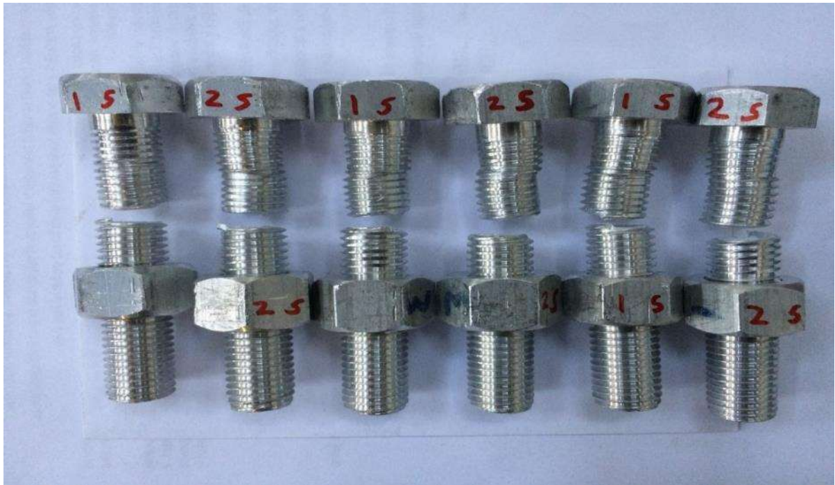
Figure 19: Failure of AA6XXX series bolts in shear at 20°C
