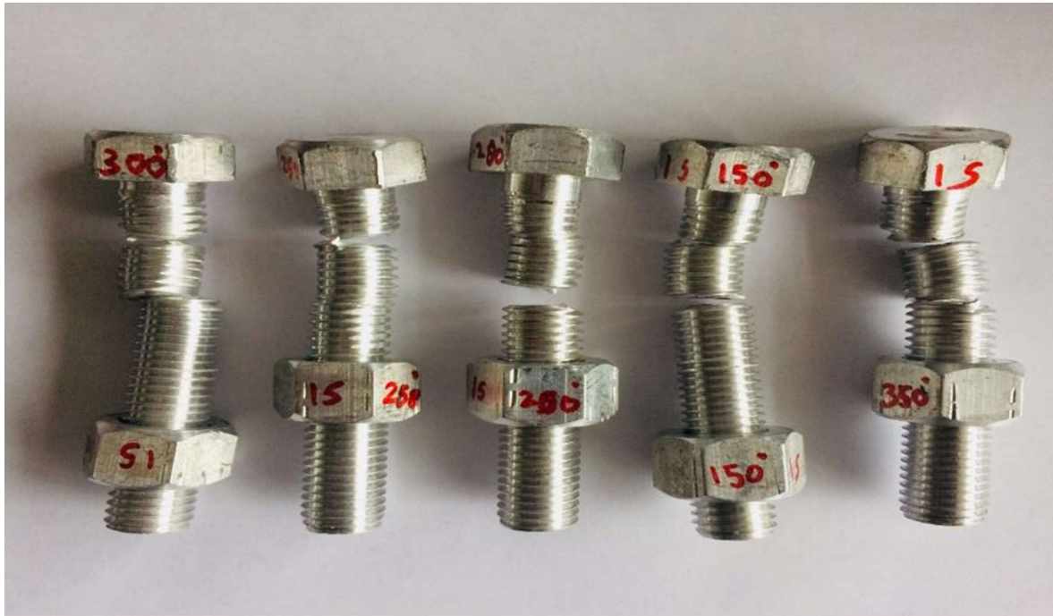
Figure 20: Failure of AA6XXX series bolts in shear at elevated temperature (150°C- 350°C)
