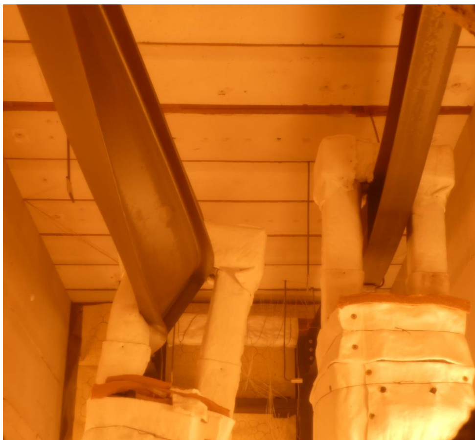
EF after 27 minutes of the test
