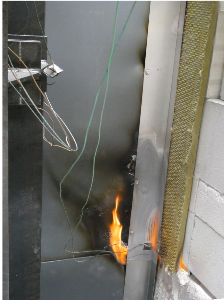
Sustained flaming of the vertical edge of the wall from 69 th minute of the test
