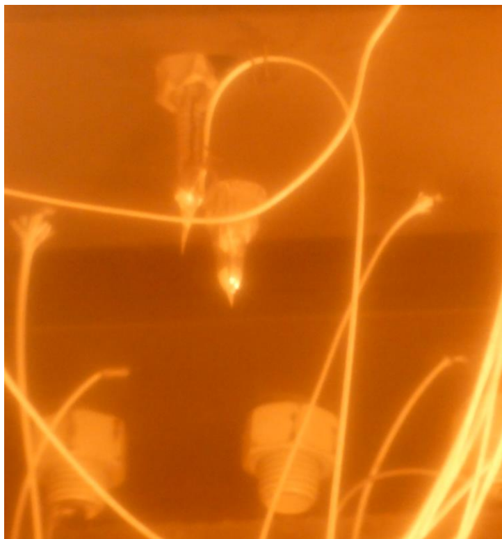
View of the fusible link No. 2 after 25 minutes of the test
