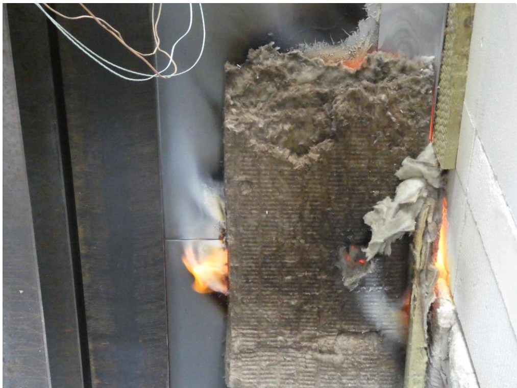
UF of the wall after 110 minutes of the test
