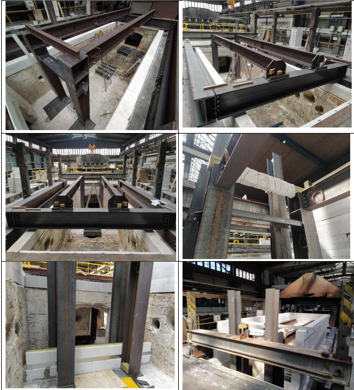
Figure 2: Manufacture and preparation of the test specimen
