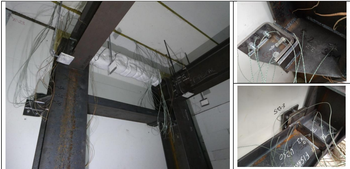
Figure 5: View of fusible systems inside the furnace
