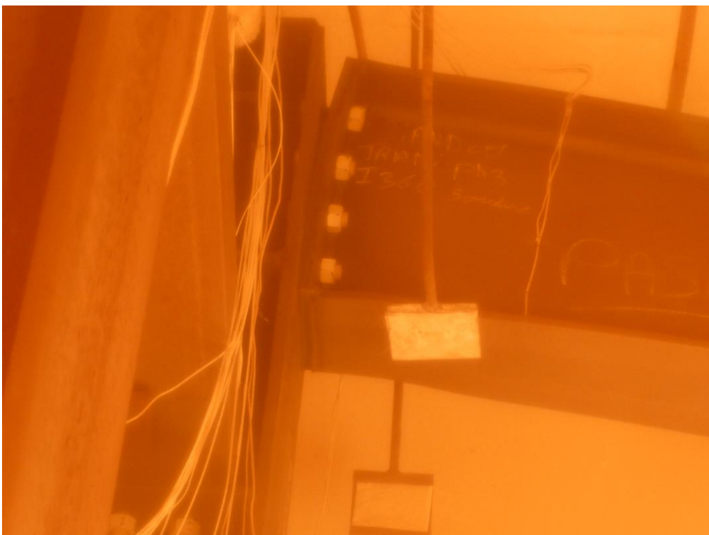
Detail of the beam to column connection of steel portal frame No. 2 after 32 minutes of the test
