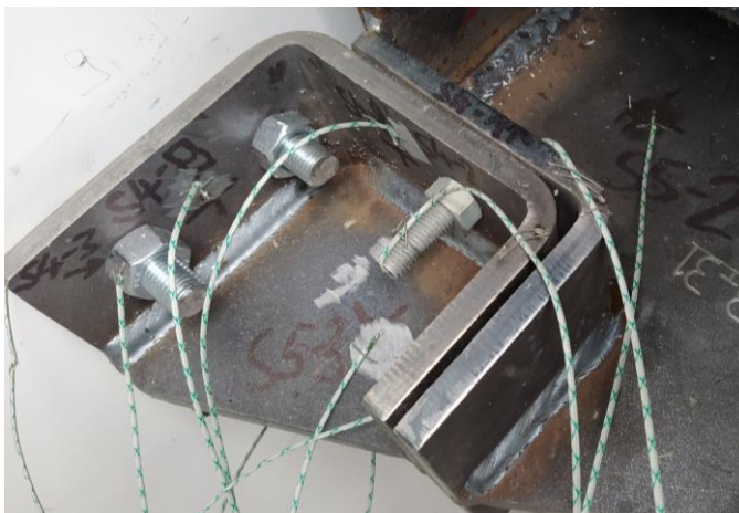
Detail of the thermocouples in the area of the fusible links
