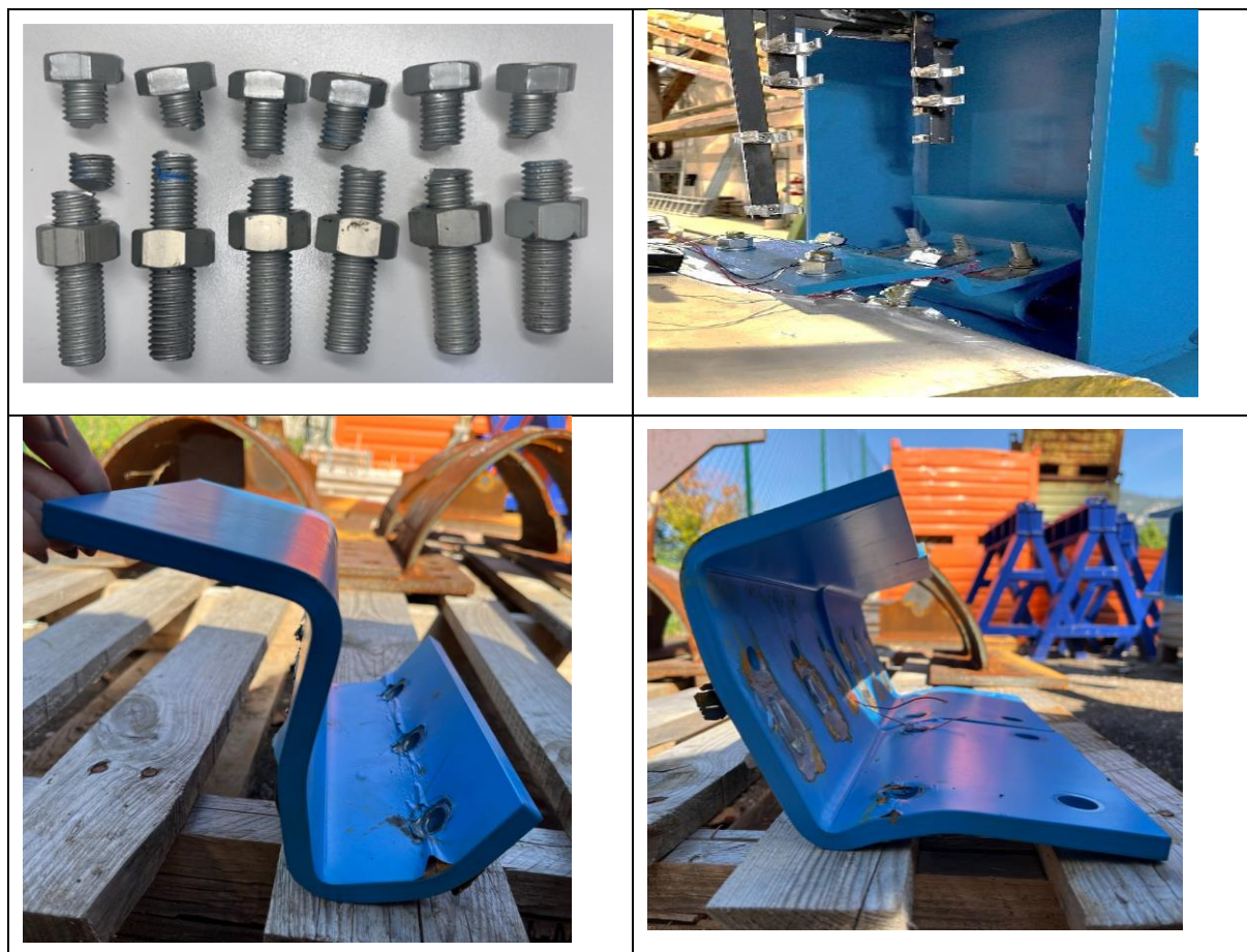
Figure 2.19: Photos of the test specimen after the test.
