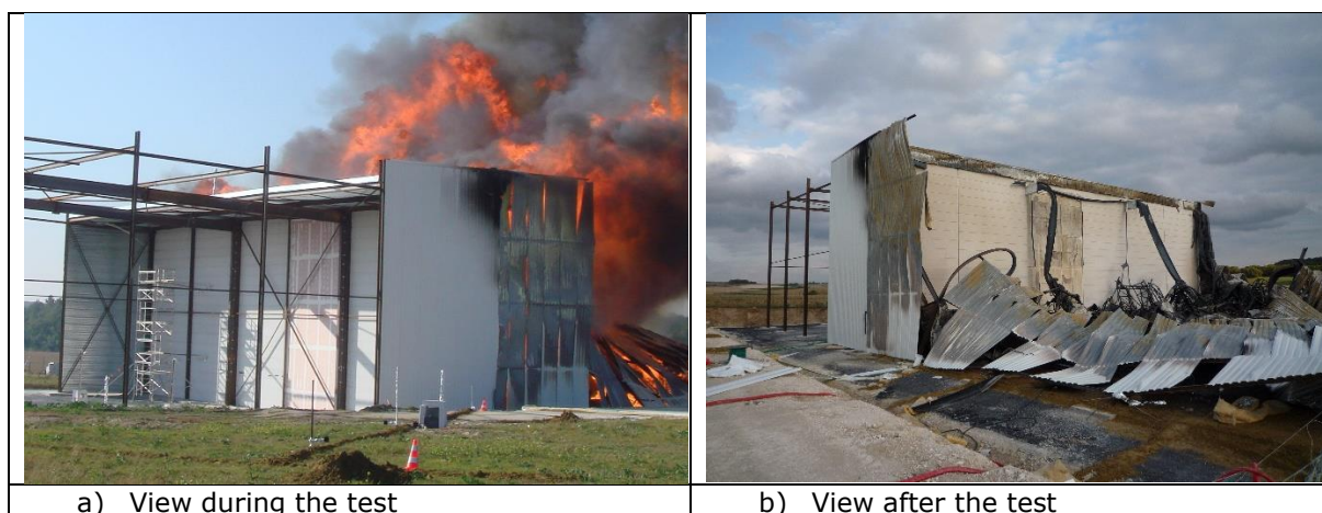
Figure 5.19: Large-scale fire test on a single-storey steel-framed building – Flumilog project
