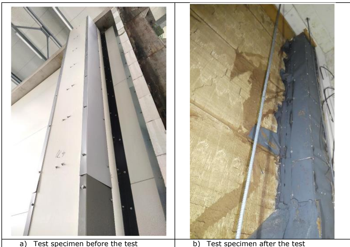
Figure 5.6: Fire test on a fire wall made with large-span sandwich panels – Fishwall project
